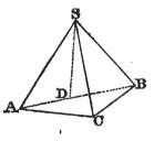
In the plane ASB make the angle BSD=BSC, draw the straight line ADB at pleasure; and having taken SC=SD, join AC, BC.
