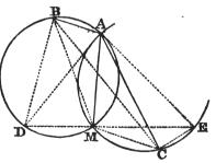
are the only ones from which AB can be seen under an angle equal to AMB; those of the arc AMC are the only ones from which AC can be seen under an angle equal to AMC; hence the point M, where those arcs intersect, is likewise the only point from which AB and AC can at once be seen under the angles AMB, AMC. We are now to calculate the position of the point M trigonometrically, from this construction.
