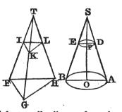
case, the vertices S and T will be equally distant from the plane of the bases, and the plane EPD produced will form in the pyramid a section IKL. Now this section IKL is equivalent to the base DE : for (287.) the bases AB, DE are to each other as the squares of the radii AO, DP, or as the squares of the altitude SO, SP; the triangles FGH, IKL (407.) are to each other as the squares of these same altitudes; hence the circles AB, DE are to each other as the
