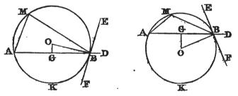
Produce AB towards D; at the point B, make the angle DBE=C; draw BO perpendicular to BE, and GO perpendicular to AB and bisecting it; and from the point O, where those perpendiculars meet, as a centre, with the distance OB, describe a circle: the required segment will be AMB.
