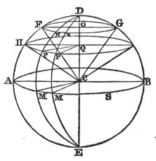
438. The *radius of a sphere* is a straight line drawn from the centre to any point of the surface; the *diameter* or *axis* is a line passing through this centre, and terminated on both sides by the surface. \*
