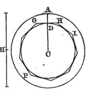
surface of a less cylinder; of the cylinder, for example, the radius of whose base is CD, and whose altitude is H.
