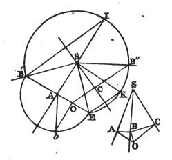
Conceive the same construction to be made as in the preceding Theorem; the angle OAB would be the angle sought. It is required to find the same angle by a plane construction, or one performed on a plane.
