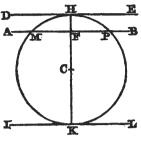
Third. If the two parallels DE, IL, are tangents, the one at H, the other at K, draw the parallel secant AB; and, from what has just been shewn, we shall have MH=HP, MK=KP; and hence the whole arc HMK=HPK. It is farther evident that each of these arcs is a semicircumference.
