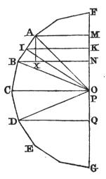
the polygonal sector AOD, will have for its measure  $\frac{2}{3}$ . OI<sup>2</sup>. (MN+NP+IQ); or,  $\frac{2}{3}$ . OI<sup>2</sup>. MQ; or,  $\frac{1}{3}$ . OI<sup>2</sup>.2MQ; or equal to a cone whose base is *surf*. OI and altitude 2MQ.
