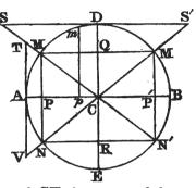
minated, is called the *tangent*, and CT the *secant* of the arc AM, or of the angle ACM.
