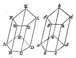
To construct this solid, let ABCDE be any polygon; then if in a plane parallel to ABC, the lines FG, GH, HI, &c. be drawn equal and parallel to the sides AB, BC, CD, &c. thus forming the polygon FGHIK equal to ABCDE; if in the next place, the vertices of the angles in the one plane be joined with the homologous vertices in the other, by straight lines, AF, BG, CH, &c., the faces ABGF, BCHG, &c. will be parallelograms, and ABCDEFGHIK, the solid so formed, will be a prism.
